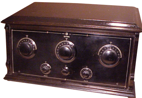
FADA (Frank Angelo D’Andrea), Model 175 – A five-tube receiver of 1925. FADA was one of the first radio manufacturers to incorporate the Hazeltine Neutrodyne circuit in their radios. FADA lasted well into the 1950’s with radio and Television products. Dave Crocker, Mashpee, MA.
